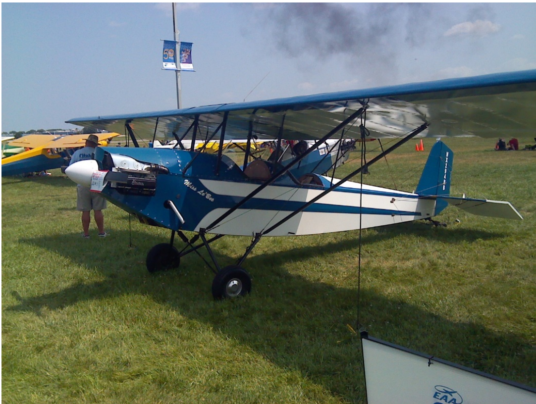
A Corvair powered Pietenpol illustrating the variety of engine options available to the do-it-yourself builder
