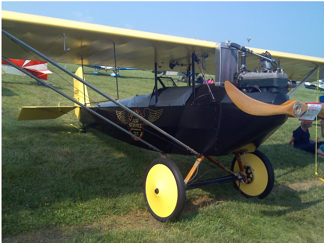
Ford Model A powered Pietenpol, it was reported to have 50HP.
