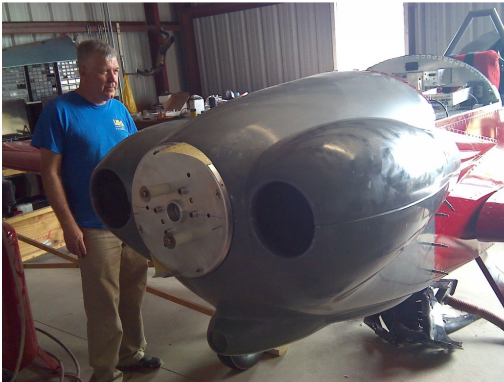
Eddie inspects the fit-up of the Cowling
