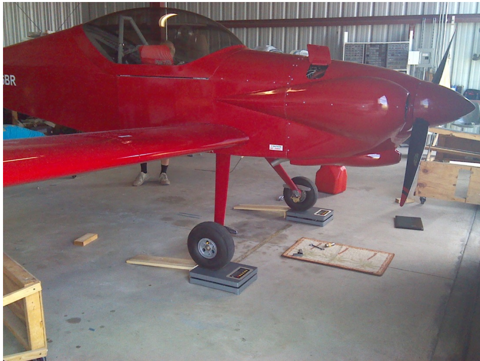
Recent Weight & Center of Gravity Determination
