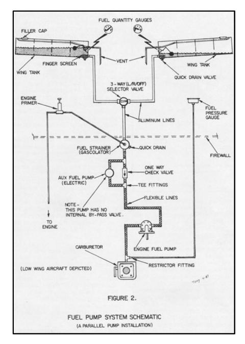
Let's consider for a moment if we had a high-wing airplane with fuel tanks in the wings. Then we could achieve *Dissimilar Redundancy* in the fuel system using the most reliable delivery method ever, gravity. Gravity is 100% reliable, and is the reason why most high wing airplanes do not need an auxiliary electric Boost Pump to achieve a high reliability system.
