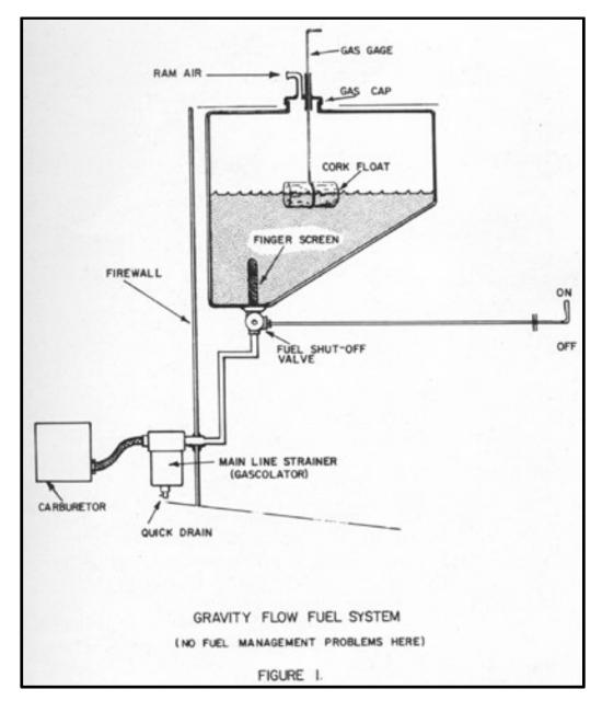
And yet, this is pretty close to what you will find in a J-3 Cub, or a Pietenpol, and we all know that both have very reliable fuel systems. This is where the whole concept of Failure Tolerance can get a little tricky and requires thoughtful consideration.
