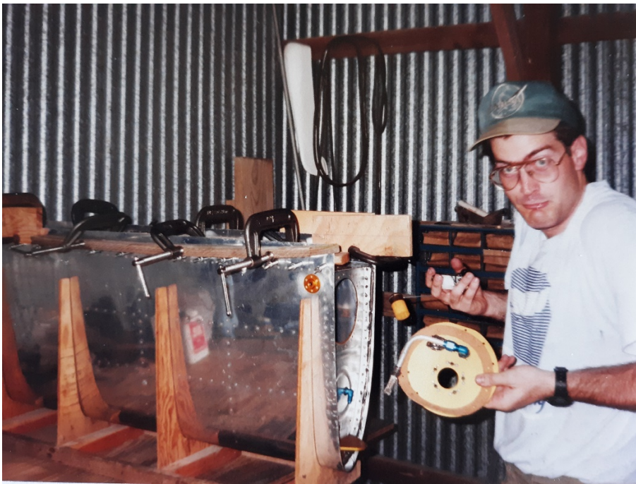
Les building the RV-4 wing tanks around mid-1998.
