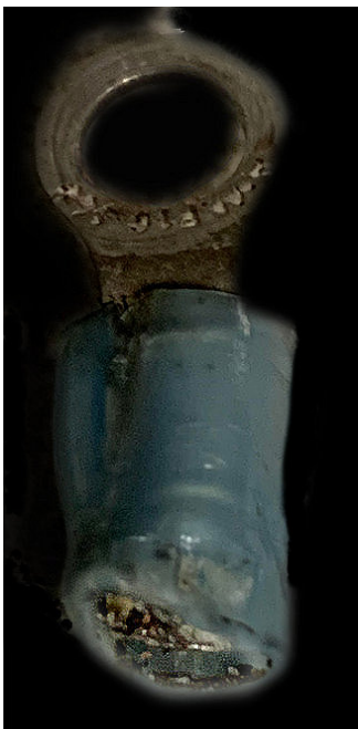
P lead terminal – wire broke off at the crimp
