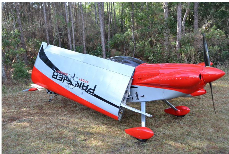
Photo: Panther prototype – only 7 feet wide with wings folded
