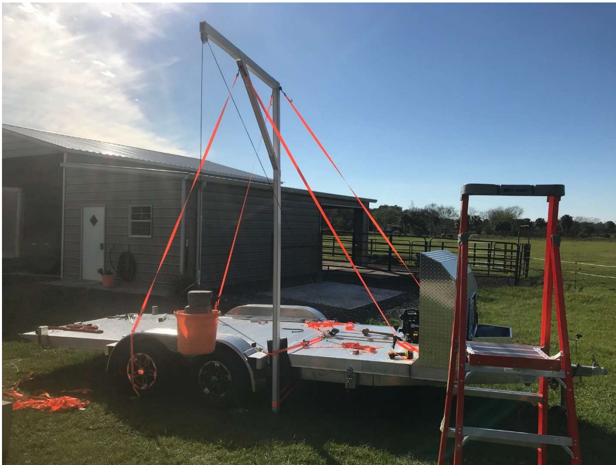
Figure 1: Load testing the rotor removal mast.
