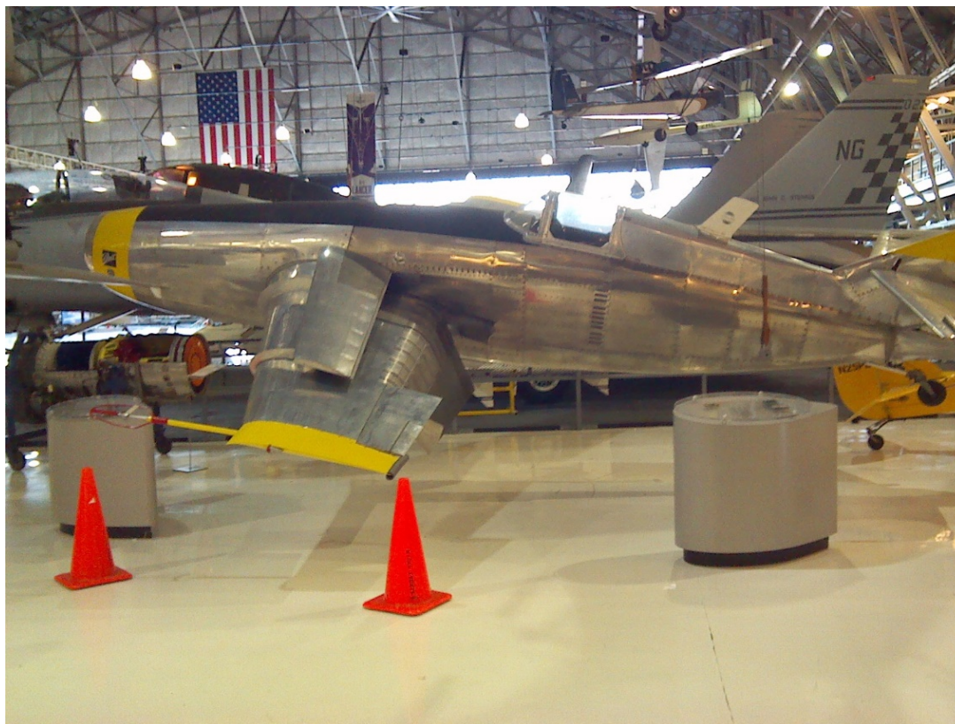
JetWing prototype high lift STOL demonstrator that test flown by Mr. Bob Hoover (Top speed of 325 knots, but able to land at only 45 knots!)
