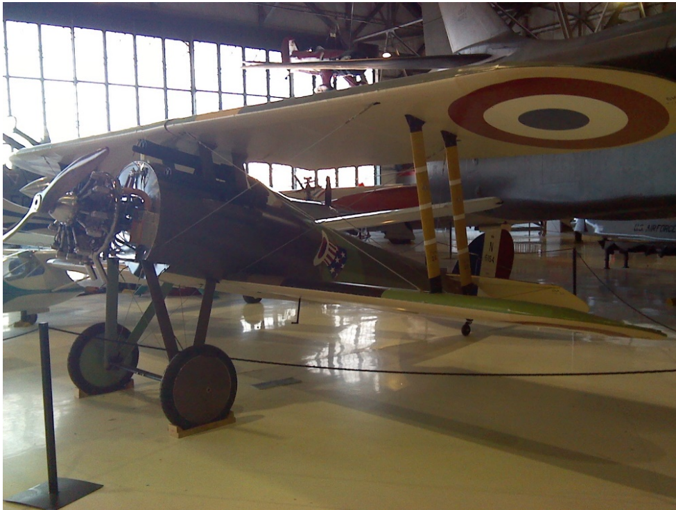
Replica WWI Nieuport fighter with a Rotec Radial engine installed
